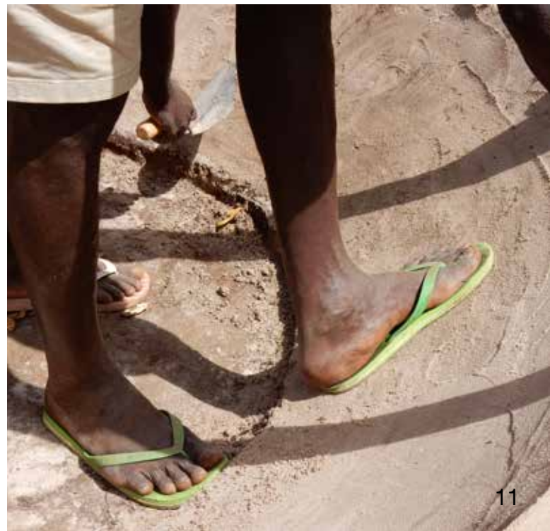
Making of the mould in wet sand in a hollow shape. The shape is for the globe-like bottom. (See page 14).
