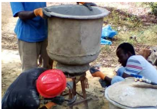
6. the roof is made on the ground, on a piece of paper of a cement bag.
