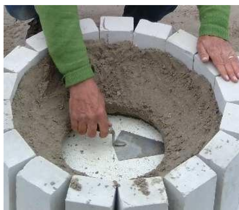
the sand mould for the foot and the bottom
